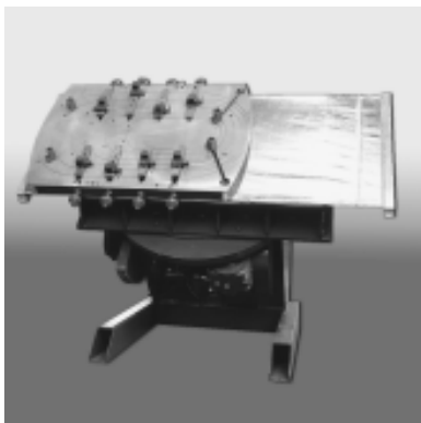
Variable speed slide table and special gripper to hold oval boxes
