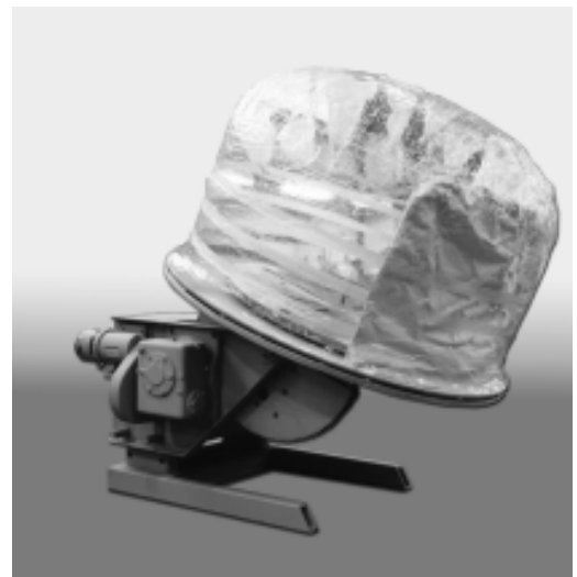
30-6 Gas Bag Positioner Designed for Inert Atmosphere Welding of Jet Engine Components.
